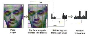
Fig.2 Examples of an LBP based facial representation
